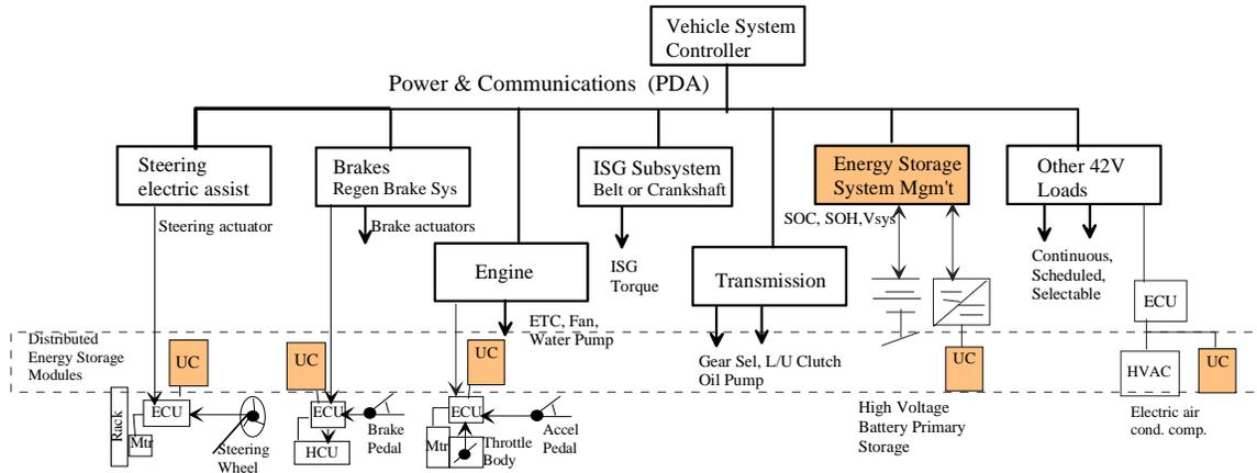
Figure 2: Distributed module architecture for vehicle safety critical and hybrid functionality
