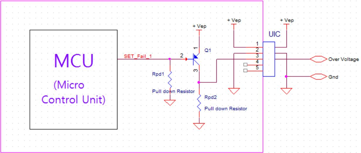
Figure 8. Diagram of Over Voltage Monitoring Circuit
