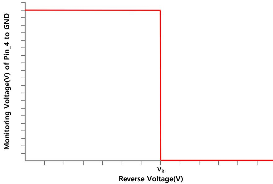
*Figure 11. Output Signal when Polarity is reversed*
