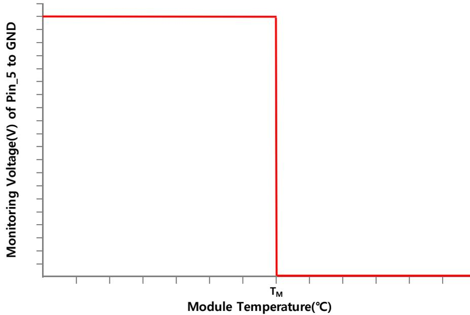
Figure 13. Output Signal of Over Temperature
