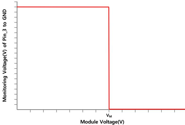
Figure 9. Over Voltage Monitoring Output Signal
