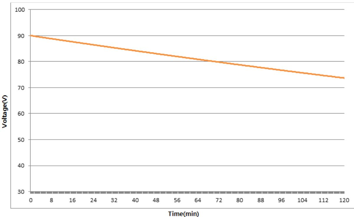
*Figure 3. Self-Discharge profile of 90V/10F module*
