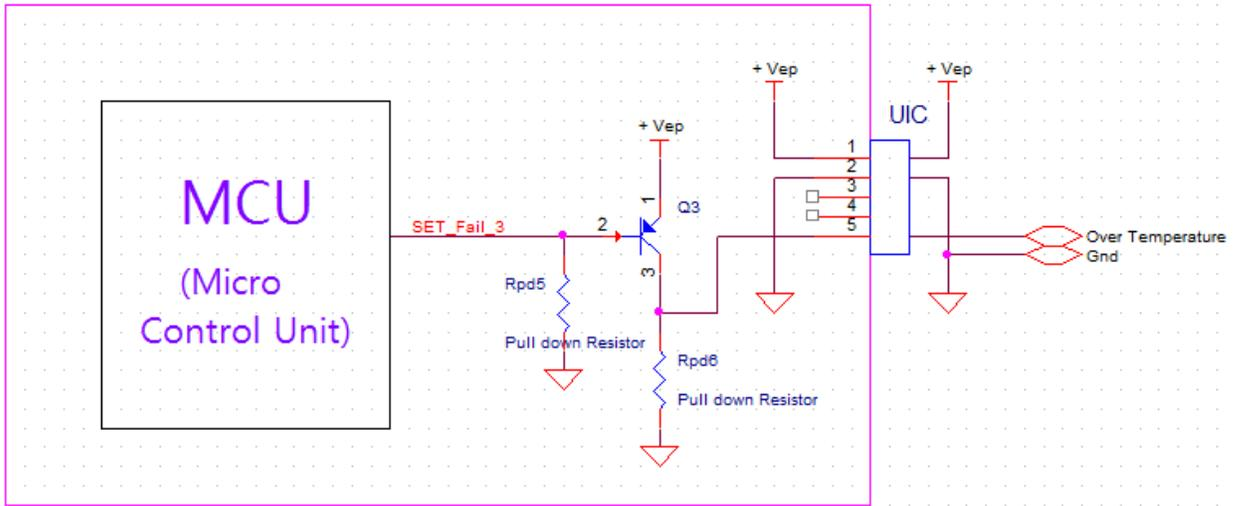
Figure 12. Diagram of Over Temperature Monitoring Circuit
