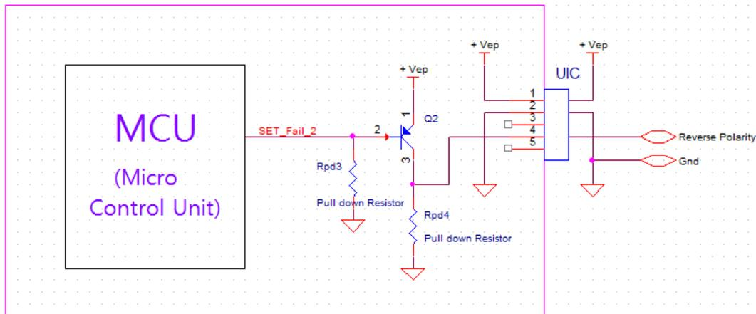
Figure 10. Diagram of Reverse Polarity Monitoring Circuit
