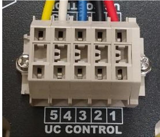
*Figure 7. Monitoring Signal Output Terminal*
