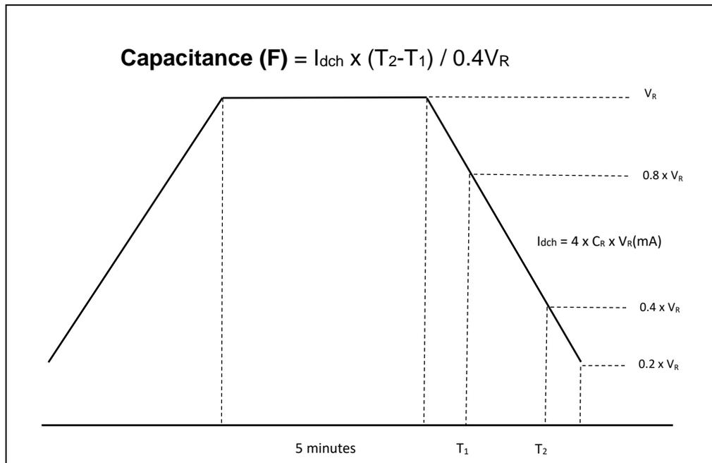
*Figure 2. Capacitance Measurement*
