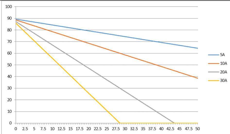
Figure 4. Constant Current Discharge Profile of 90V/10F
