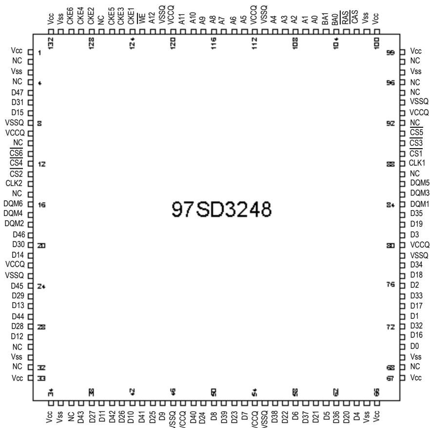
The 97SD3248 Consists of 6, 8-Meg X 8-Bit X 4-Banks, die.
