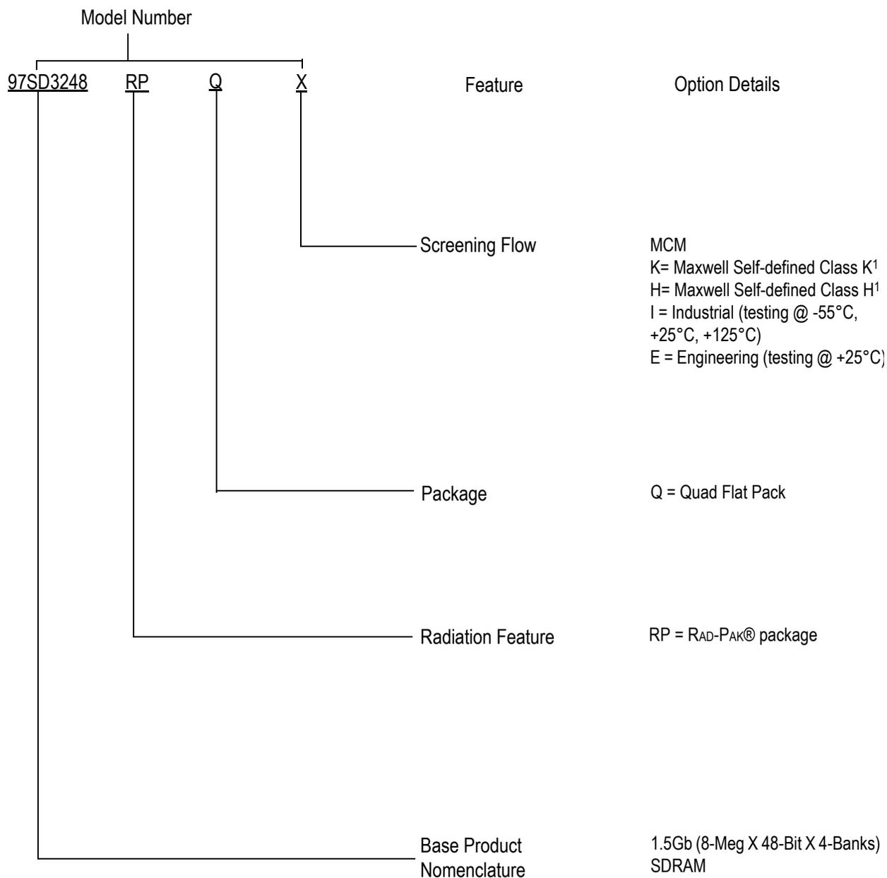
1) Products are manufactured and screened to Maxwell Technologies self-defined Class H and K flows in a MIL-PRF-38535 qualified facility.
