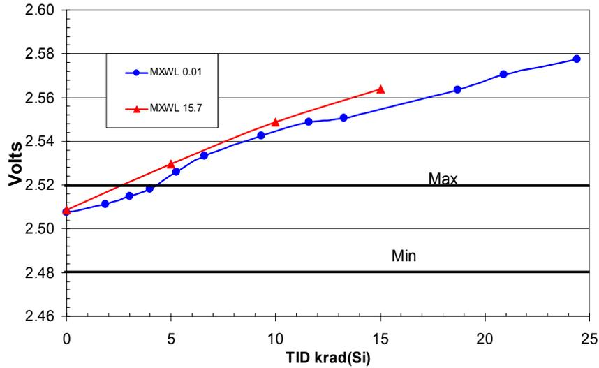
Figure 4. 7805 Voltage reference drift for two dose rates
