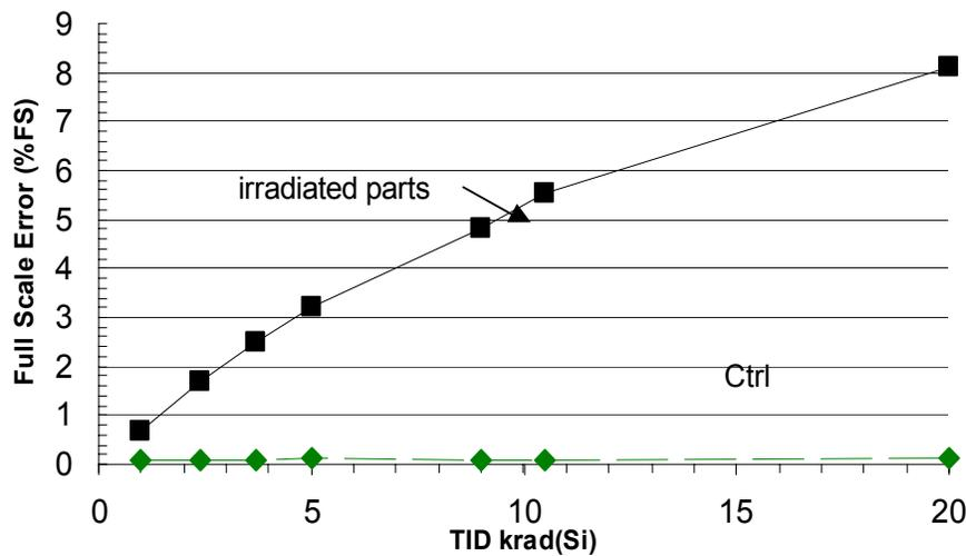
Figure 7. 7809LPRP Unipolar Full Scale Error TID degradation.
