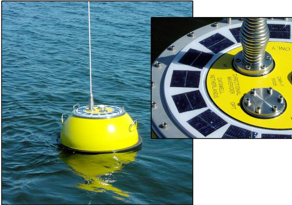
The Waverider buoy, showing the solar cells on top of the stainless steel hatch cover, protected by a layer of polycarbonate.
