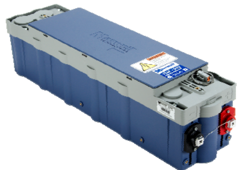
Figure 1. 56V Module which can work in series connection up to 750V. Each module can nominally support 10kW for 15 seconds.
