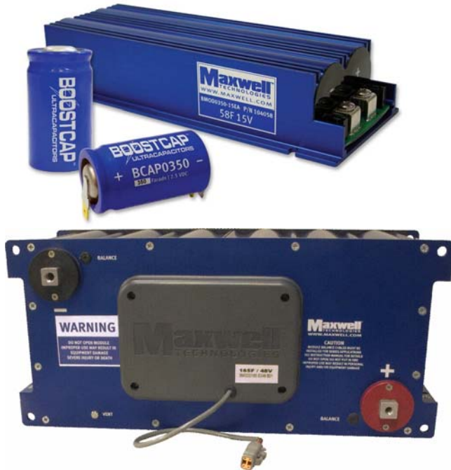
Figure 6 Energy D Cell Ultracapacitor Cell (350F, 2.5V, 3.2mΩ, 60g, Pml=5.6kW/kg) and Module (left), and 48V Module (right) Designed for Heavy Transportation Applications
