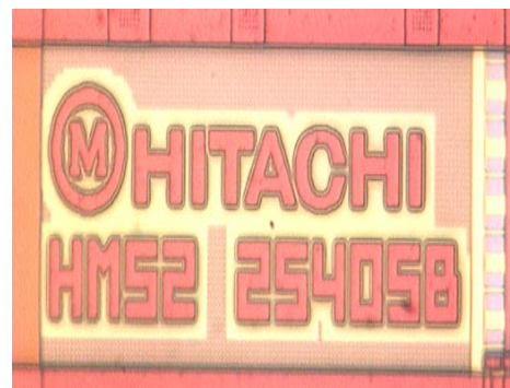
Figure 5. Die part marking
