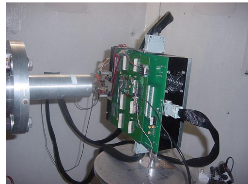
Figure 2. SDRAM test board irradiated at Texas A&M's Cyclotron
