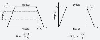
where C is the capacitance (F); I is the absolute value of the discharge current (A); V<sub>B</sub> is the rated voltage (V);
