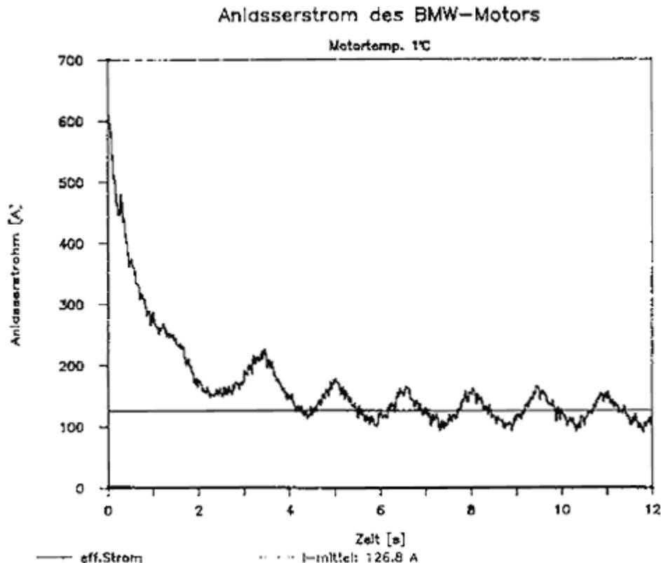
Figure 3: Current of a starter (BMW) at 1°C [2]
