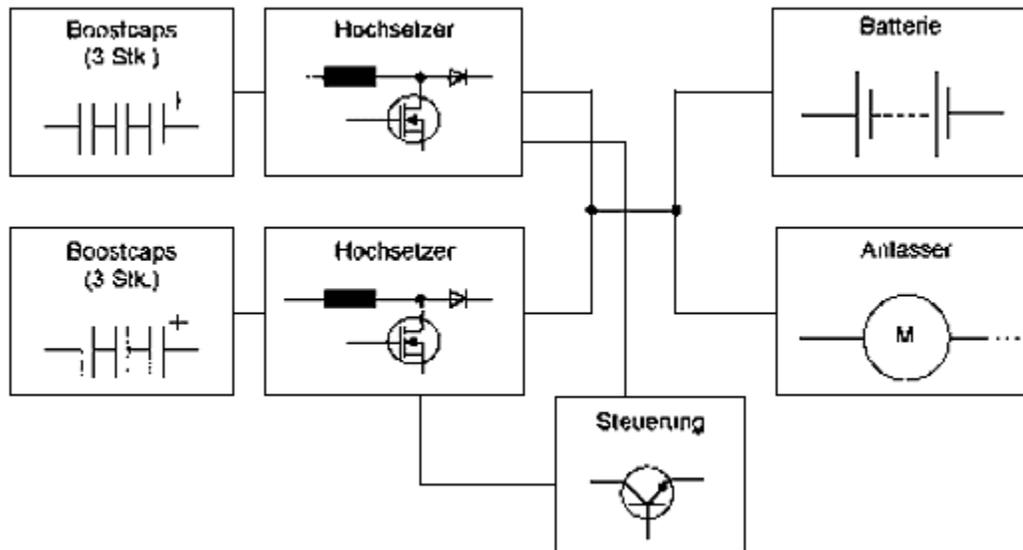
Figure 4: Block diagram of the starter unit
