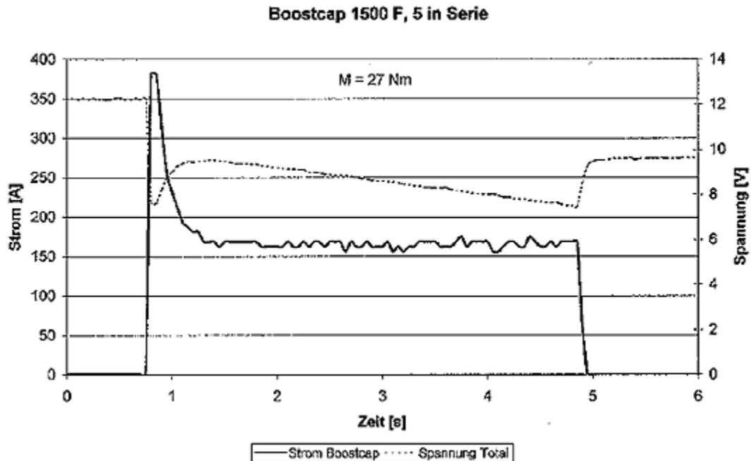
Figure 5: Current and voltage of a 1 kW starter motor measured on the test bench of HTA Biel [4]
